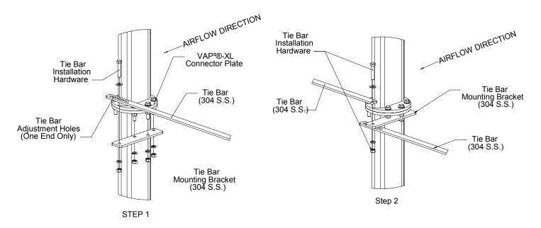
Figure 6 VAP<sup>3</sup>®-XL Tie Bar Installation
